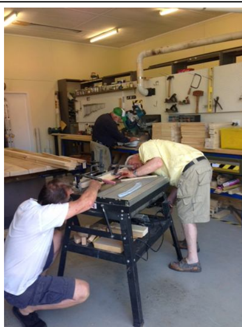
Joe and Jack set up the router table whilst John cuts blocks on the radial arm saw.
